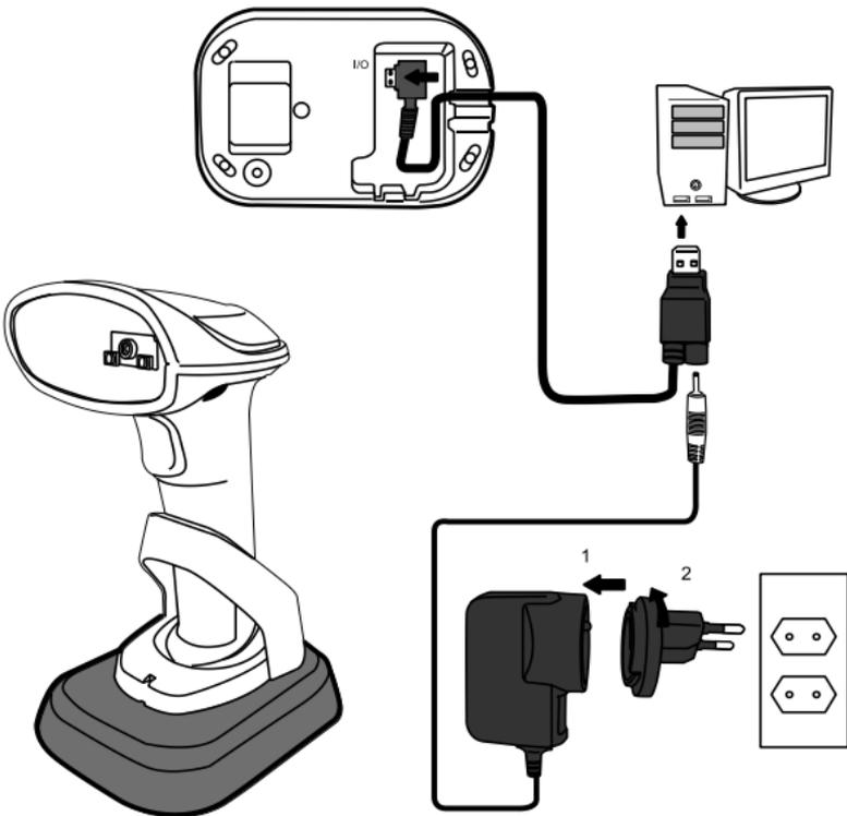
1. Connect the USB or the RS-232 cable to your cradle. Lay the cable into the notch on the cradle edge.
