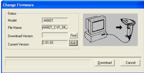
11. Click **Find** to load the firmware file. The firmware version in this file needs to be different from the current firmware version of your cradle. After loading the file, click **Download** to update the firmware of your cradle.
