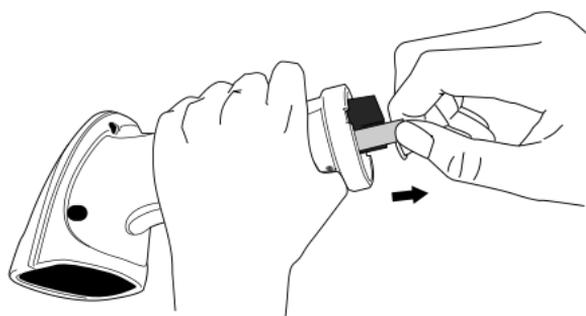
4. Insert the new battery into your scanner in the direction of the arrow printed on the battery.
