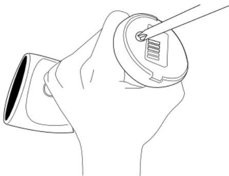
2. Remove the battery cap.
