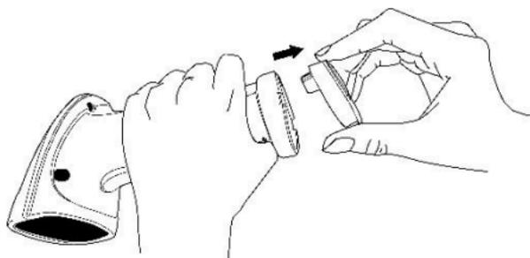
3. Pinch the tape at the top of the battery and pull the battery out.
